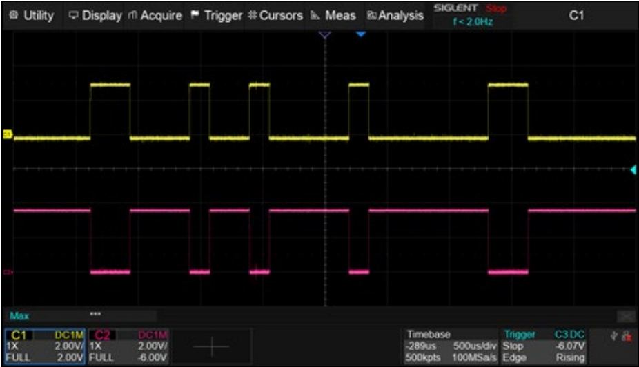
Fig 2: PWM signal pulse generated by TMS320F28335 DSP for inverter control.
