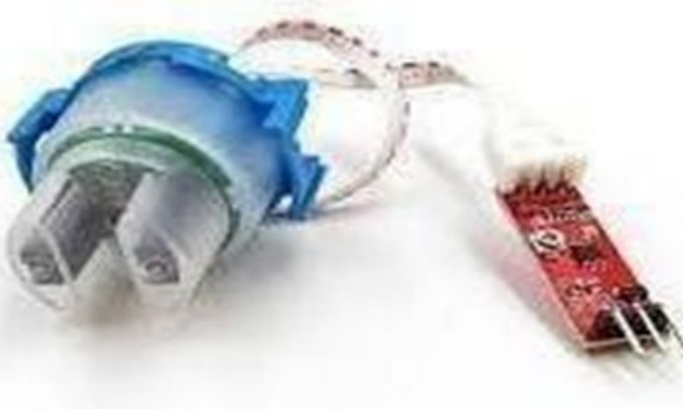
Fig 2: Turbidity sensor with module
