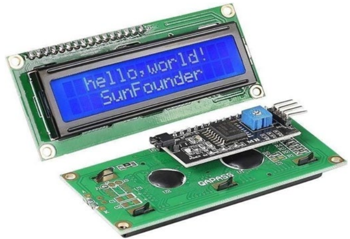
Fig 3: LCD 16x2 with I2C Module
