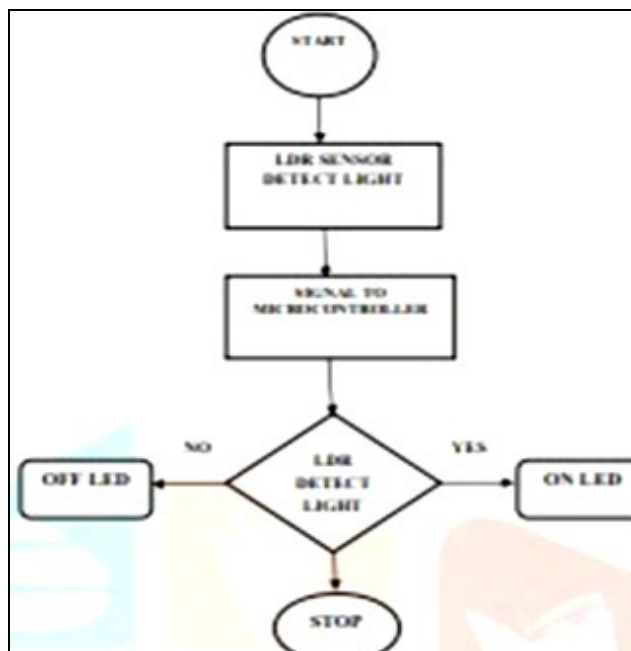
Fig 7: Flow chart explaining working of LDR sensor
