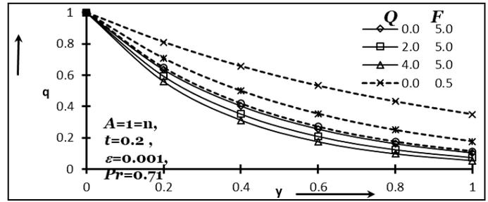
Fig 5: Temperature distribution for Q and F
