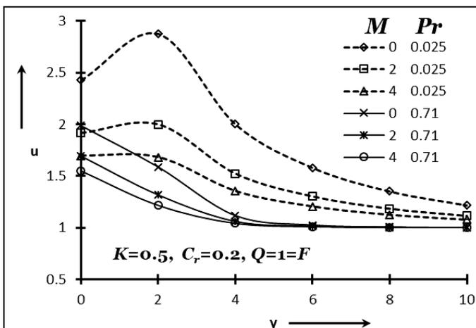
**Fig 1:** Velocity distribution for M and Pr
