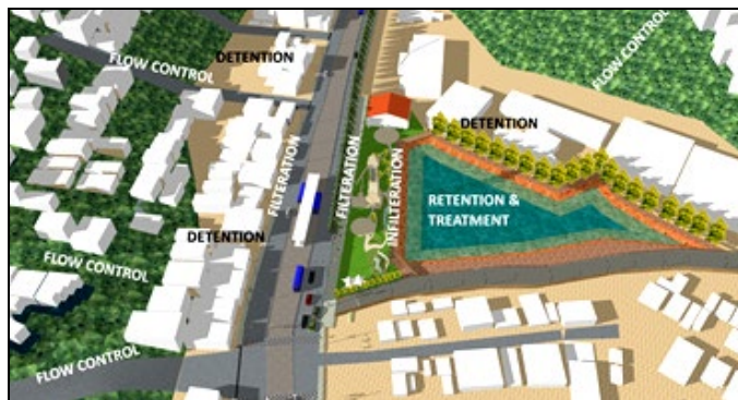
Fig 25: The process of flow control, Detention, Retention, Filtration, infiltration and Treatment in the proposal.
