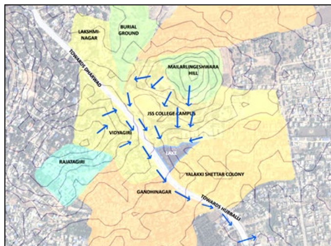
Fig 9: Contour map showing the slopes and arrows showing present condition of flow of storm water. (Contours map generated in QGIS)
