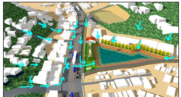
Fig 26: Make proper way for rain water surface runoff and direct it towards the pond by cleaning and removing the debris from its way. The catchment area in the surrounding hilly areas provides better supply of rain water to this pond. (3D view by author).
