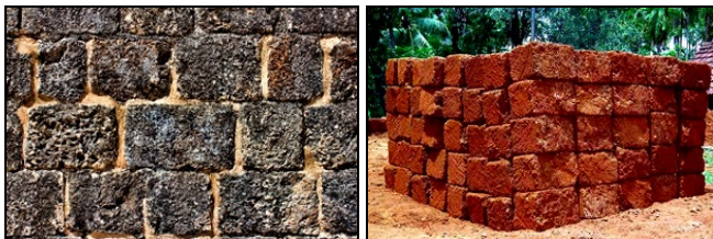
Fig 2: Construction Material as Natural Laterite Stone as a resource in India for thermal cooling.
