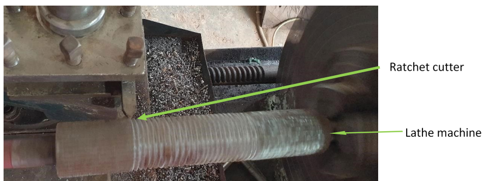
Fig 19: Development of roller in lathe machine
