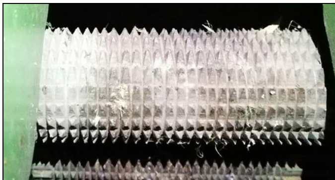
Fig 23: Teeth arrangement in working roller
